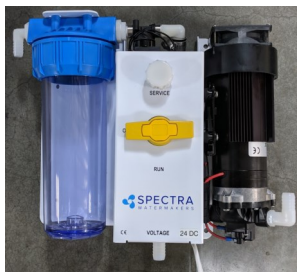
Service valve OFF, in FLUSH position
