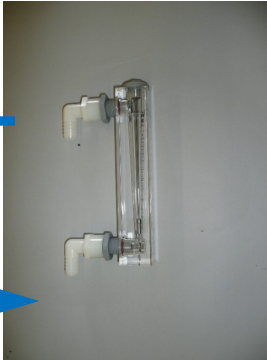
Feed Flow Meter
